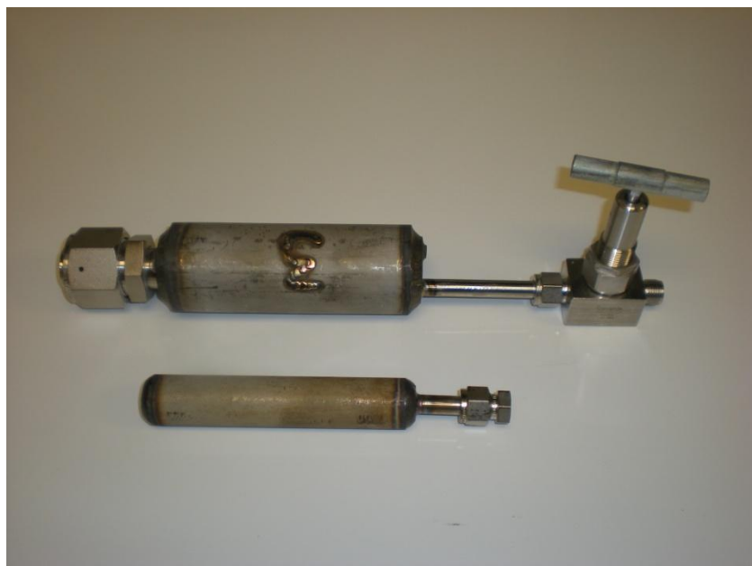
Figure 1: Showcasing the 1" (bottom) and 2" (top) heavy duty cell sizes
